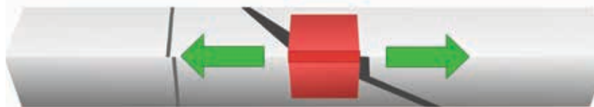
Each time across, a vacuum sucks a page from one side to the other.
