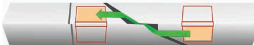
The pages are scanned as they travel across two imaging sensors.
